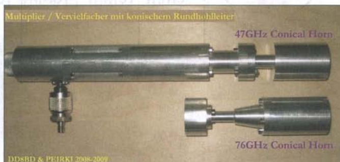
Fig. 9: Multiplier with conical horns for 47GHz and 76GHz
