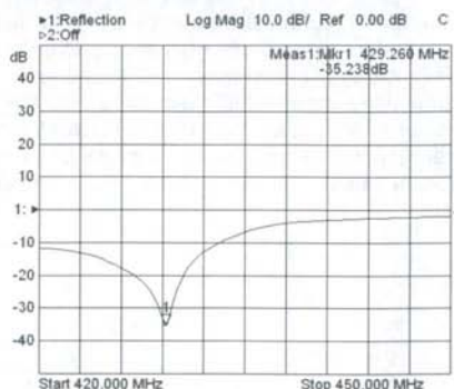
Chart 4: 70-5 on 25 x 25 mm aluminium boom, BC = 3.5 + 3.5 = 7.0 mm
