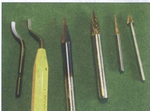
Fig. 12: Universal countersinks and conical milling cutters for circular WG adapters
