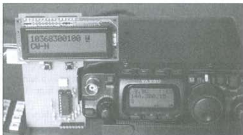
Fig. 1: Frequency Reader in operation with a test L.O. of 10224000.0 kHz. All the circuit fits under the display. The 10x5cm board also holds the keypad option (see text).
