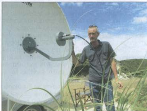
ZL1TPH and his dish with 23/13cm loop feed
