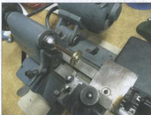
Fig. 6: Checking a WG & flange for squareness
