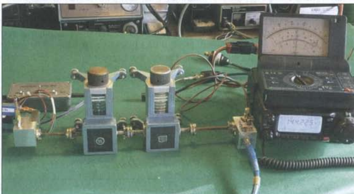
Fig. 15: Measurement setup for 122 GHz with two 50 dB attenuators reading to 1/10 dB
