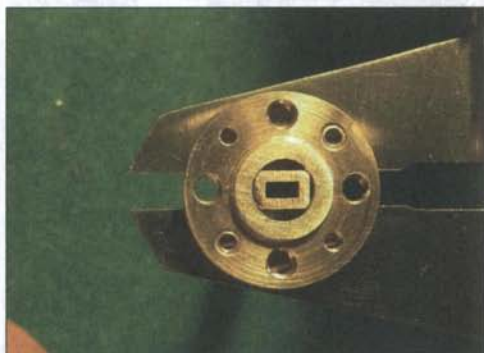
Fig. 5: Checking angular positioning with a calliper
