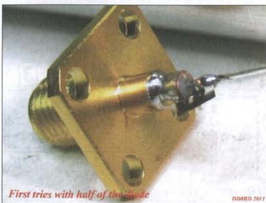
Fig. 7: BAT15-099 – just one half is soldered here
