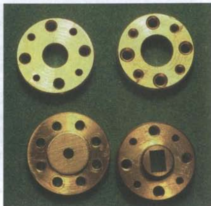
Fig. 3: DIY drilled flanges for WR 19, WR 12 and WR 4, with a professional WG387 flange
