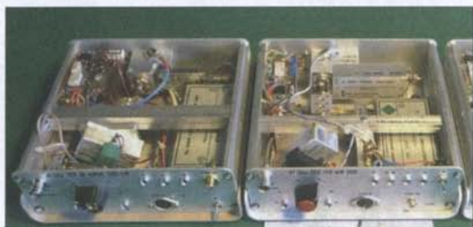
Fig. 2: Completed transverters for 47 GHz and 76 GHz with mechanical changeover
