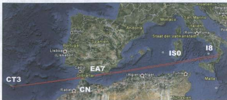
2m Tropo QSOs from CT3HF (IM12OP) to IW8QQJ (JM88GW, 3069km) and IW8QOT (JM88BR, 3032km) on August 24 th 1999
