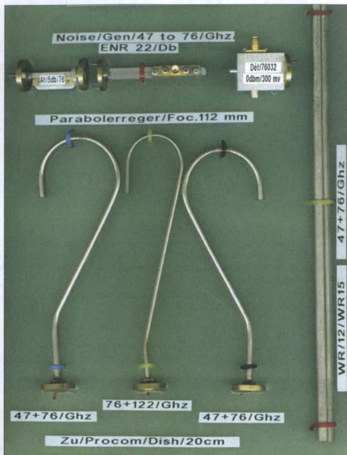
Fig. 1: Top, from left: 1. Variable attenuator 60-90GHz. - 2. Noise generator 47-120GHz, 22dB ENR. 3. Detector 47-76GHz, 0dBm = 300mV. Below: 4. WG feed 47-76GHz 5. WG feed 76-122GHz. Right: Waveguides WR12 and WR15
