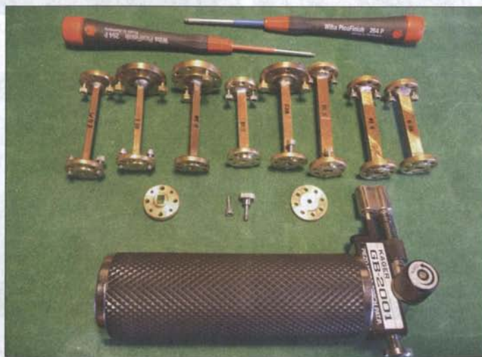
Fig. 11: Completed WGs with flanges, similar to WG387 and WG383, with flange connecting screws and screwdrivers for inner hexagon
