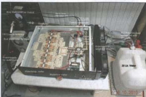
PA3DZL SSPA 1296 8xXRF286S water cooled
