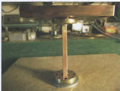
Fig. 10: Upper flange is already soldered, and now protected from melting by a copper plate
